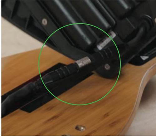
*Battery pack connector clip in place*
