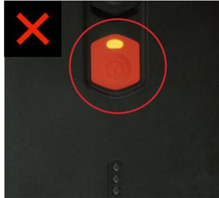
*Battery pack not properly connected*
