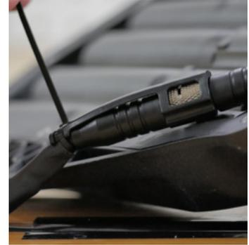
*Tighten down zip tie to close the loop and cut excess length away*
