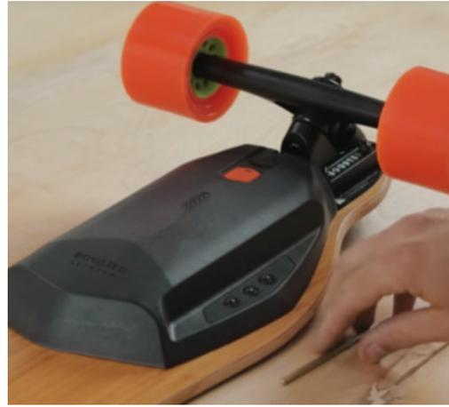
Battery pack in proper placement
