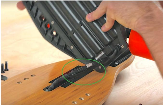
*Battery pack connector clip in place*
