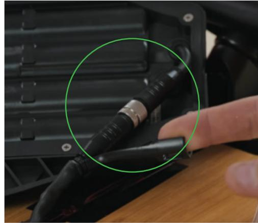
*Unclipped battery pack connector clip*
